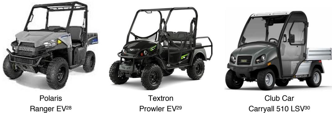
Whichever vehicle is chosen, it would need some modification—the Polaris or Textron would need a cab enclosure; the Club Car would need a raised suspension and off-road wheels.
