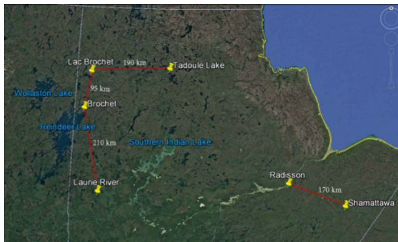
Figure 20 –Proposed Transmission Lines to Manitoba's Off-Grid Communities
