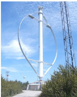
Figure 24 – Example of a vertical axis wind turbine
