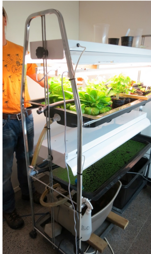
Figure 29: Vertical Aquaponics System
