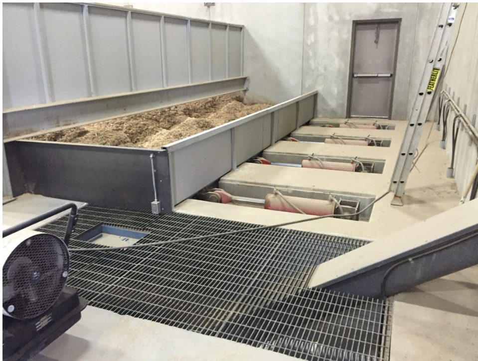
Figure 72. Pistons & Start of Auger System at Front of Walking Floor
